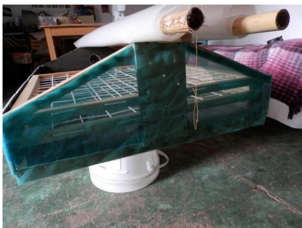
The frame to which the mosquito net is attached and which carries the ‘gable’ of the dryer.
