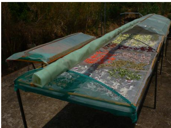
A 5m x 1,2m model filled with vegetables (Plastic film is open for the picture).
