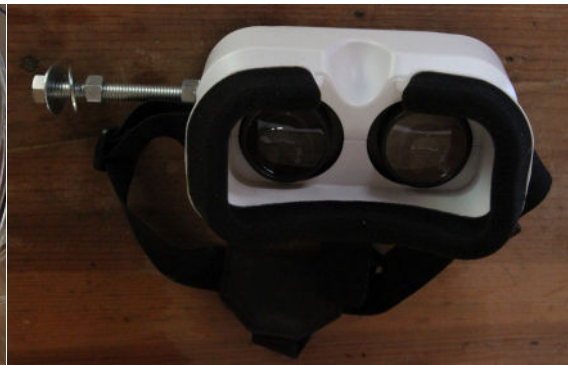
VR glasses with a threaded rod to which the bundles of fibre optic cables can be attached.
