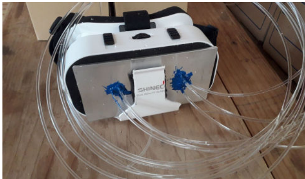
The aluminium plate with glued-in glass fibres in the VR glasses.
