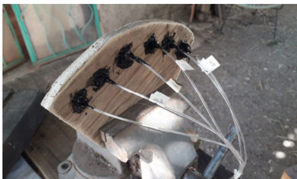
The glass fibres are glued into the controller.
