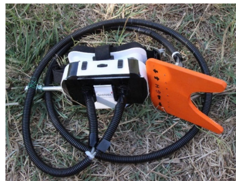
This picture shows how the fibre optic bundles are protected against light: From the side of the glasses, first 10 cm of the left and right fibres in separate sheaths, then all fibres together until right before the controller.
