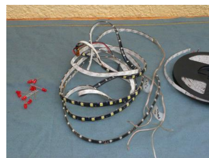
LED strips (plus some single LEDs on the left).
