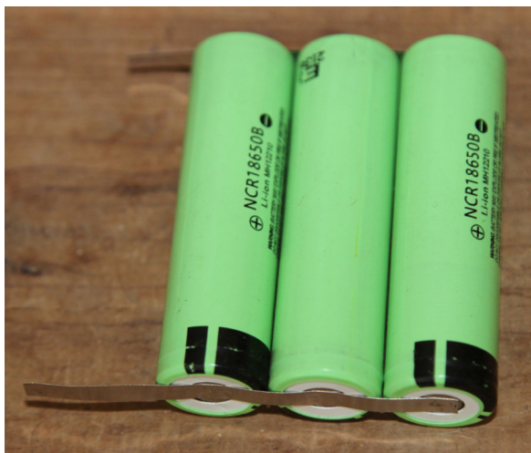
A "spot welder" can solder nickel strips to rechargeable batteries without overheating them.
