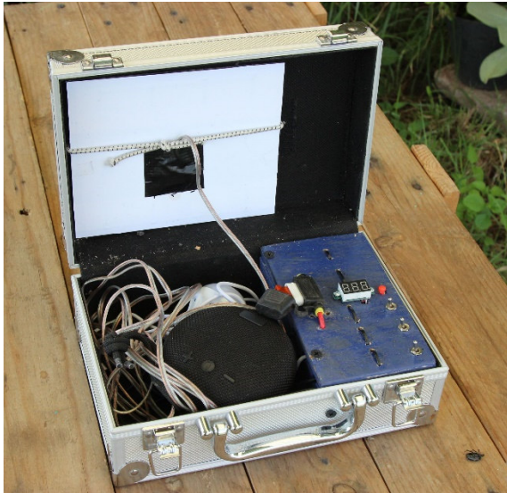
The USB solar suitcase with stowed panel, speaker and cables.
