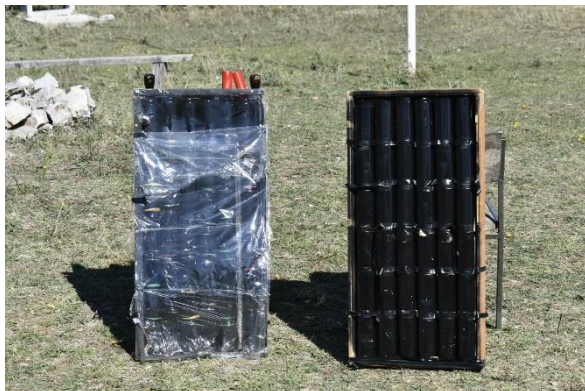
Figure 29: A self-made solar collector with and without a plastic cover against the wind, August 2022
