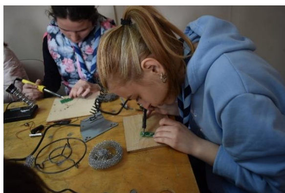
Figure 10: Soldering cables to the main board to close the circuit and make the lamps work, April 2022
